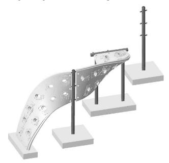
STEP #8: Using the same technique as was used in the previous step, attach the remaining Aztec Plastic Panel to the Vertical Connecting Post as well as the Horizontal Connecting Post. Secure using bolt caps, bolts, washers and nuts.
