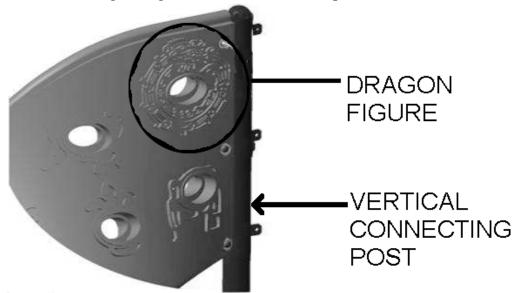
STEP #6: Spot area for Horizontal Connecting Post. Area should resemble picture below. Approximate height of the hole on lower tab on the main post to the top of the safety surfacing is 47"
